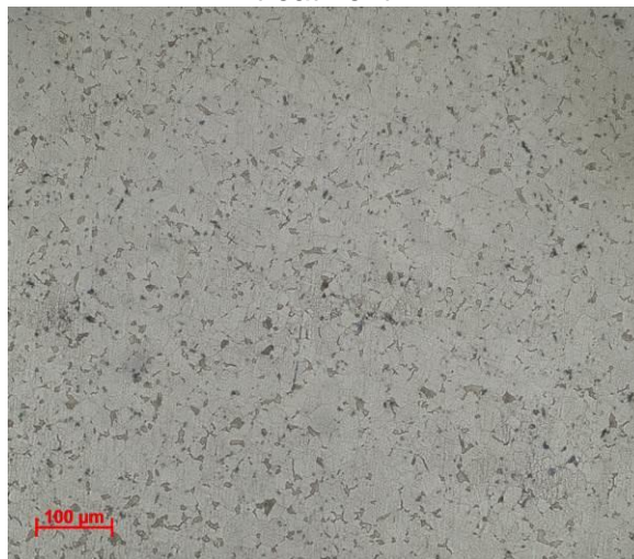
Figure 1 - Optical microscope 200x magnification – SAE 1020 carbon steel without heat treatment.
