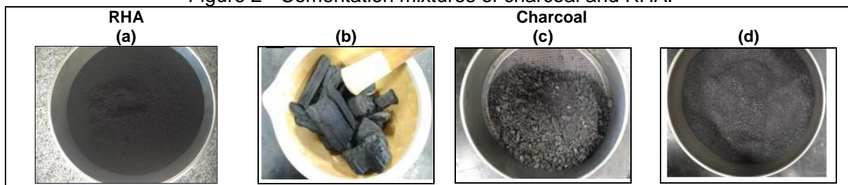
Figure 2 - Cementation mixtures of charcoal and RHA.
